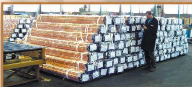
packaging copper tubes in bundles
